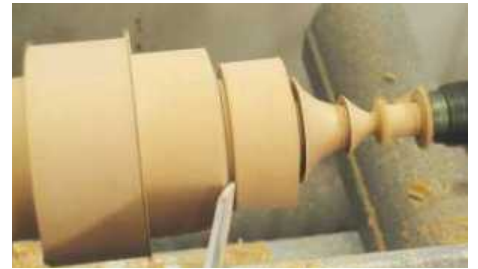
▲ Pic.3 Make a slicing cut with the 3mm parting tool, with the point cutting above centre. If the tool starts to bind, make a relief cut to one side
